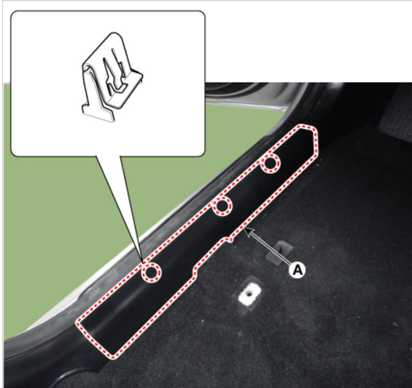
2. Remove the hood latch release handle (A).
