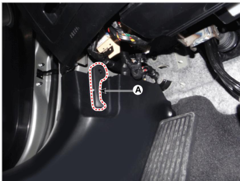
3. Carefully remove the front door body side weather strip.
